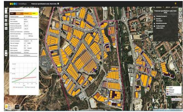
Web tool for consulting the photovoltaic potential of the roofs by ICGC.
