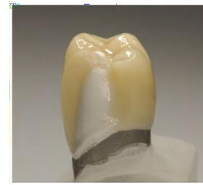
Figure 4: Cohesive fracture of a specimen from layering technique. (Beuer)
